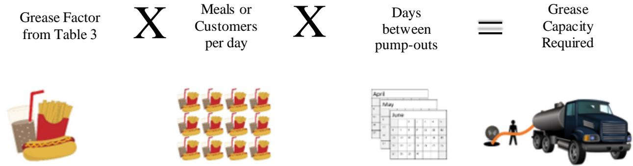
To determine the correct grease factor, using Table 3, select the menu type (1 through 30), then the correct column (A through D) for whether there is a fryer and whether the establishment uses disposable or washable plates, glasses, knives, forks and spoons (flatware).
